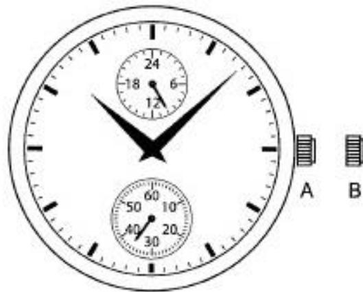
1. Pull the crown out to First Position (B) and turn Clockwise or Anti Clockwise to set time, making sure the hand on the 24 hour dial is set correctly.
